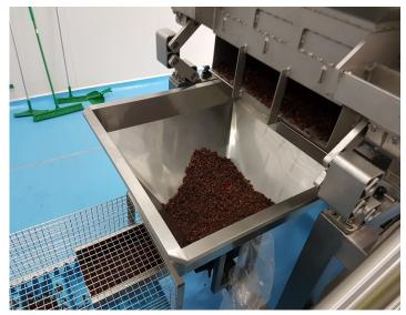
A Stainless steel construction. The Industrial Power Sieve uses Swiss vibration mount and Itatlian vibromotors to transfer up to 2 Tonnes of vibration force to the product. The Industrial Power Sieve also includes a fully automated feeding system to work in with the packaging machinery line.
